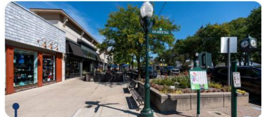
The planter box is used to separate the automobile traffic from the main street pedestrian zone.
