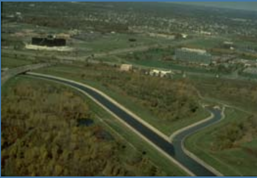
Urban: The Rouge River is highly urbanized near its mouth and has been lined with concrete to prevent flooding in downstream communities.
